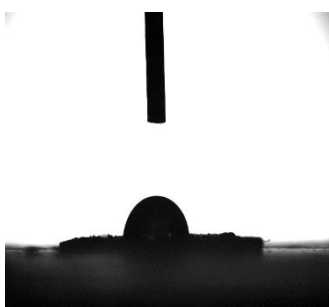
Figure 6: Contact Angle Measurement. The water droplet sitting on the surface of the dried nanoparticle film suggests a measurement of the contact angle. The contact angle measurement indicates a 42.3^\circ angle. This confirms a hydrophilic character which is conducive to better dispersion in water and also better interaction with the bio membranes, which is important for the antimicrobial functions.
