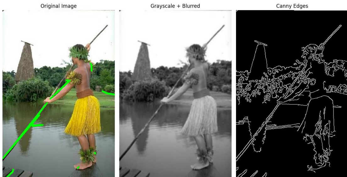
Fig 2. a) Input image b) Grayscale and Blurred c) Canny Edges
